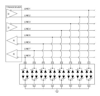
Figure1. Bidirectional Common-Mode Protection
