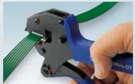
3. Bring the device plug and flat-ribbon conductor into contact using the plier.
