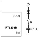
Figure 5. External Bootstrap Diode and BOOT Capacitor Series Resistor
