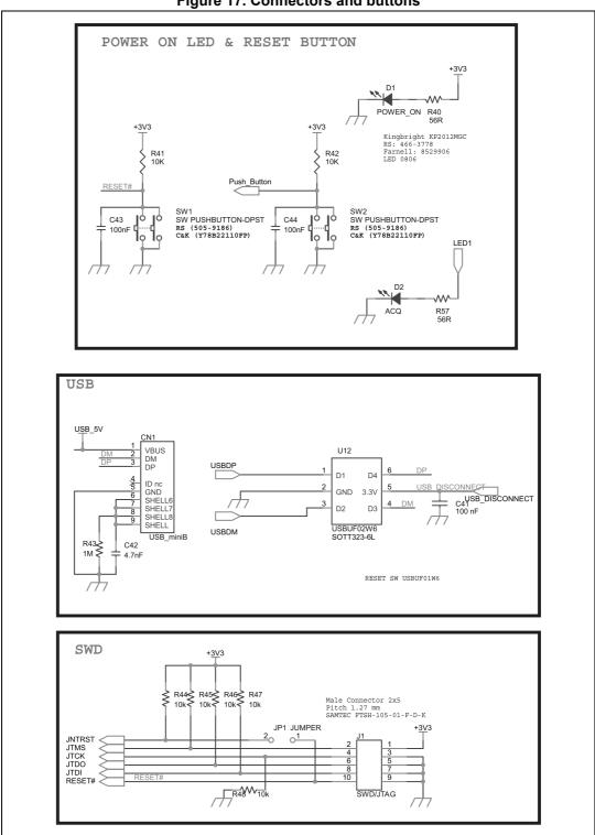
Figure 17. Connectors and buttons
