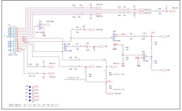
Figure 8. ECG connectors
