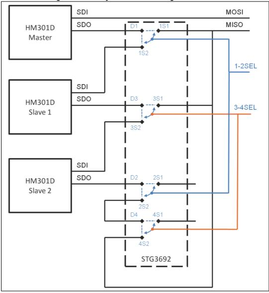
Figure 7. SPI daisy chain routed through the STG3692
