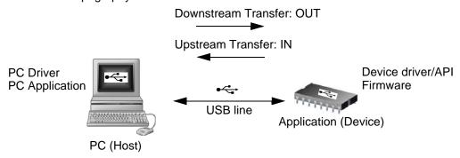
The USB used to transmit information has the following configuration:
