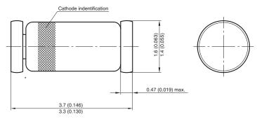
\* The gap between plug and glass can be either on cathode or anode side
