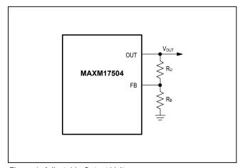
Figure 1. Adjustable Output Voltage
