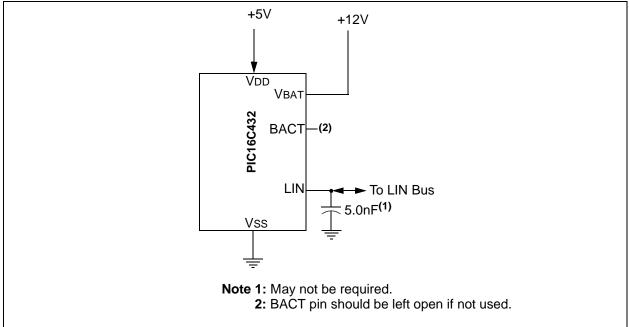
A new figure has been added to show LIN Bus configuration using Wake-up interrupt, Figure 6-3:
