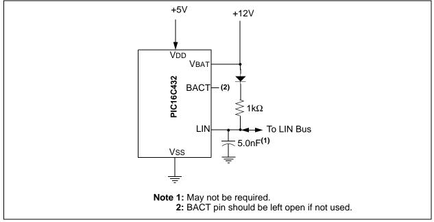
A new figure has been added to show LIN Bus slave configuration, Figure 6-2:
