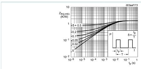
Transient thermal impedance from junction to mounting base as a function of pulse duration Fig. 5.
