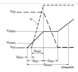
Fig. 14. Gate charge waveform definitions
