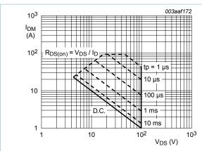
$T_{mb}$  = 25 °C;  $I_{DM}$  is single pulse
