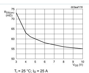
Fig. 7. Drain-source on-state resistance as a function
