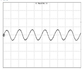
**Figure 11:** Input Terminal Ripple Current, i<sub>c</sub>, at full rated output current and nominal input voltage with 12μH source impedance and 33μF electrolytic capacitor (500 mA/div, 2us/div).
