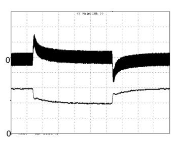
**Figure 9:** Output voltage response to step-change in load current (75%-50%-75% of lo, max; di/dt =  $1A/\mu s$ ). Load cap:  $330\mu F$ ,  $35m\Omega$  ESR solid electrolytic capacitor and  $1\mu F$  ceramic capacitor. Top Trace: Vout (100mV/div, 200us/div), Bottom Trace: I out (3.75A/div). Scope measurement should be made using a BNC cable (length shorter than 20 inches). Position the load between 51 mm to 76 mm (2 inches to 3 inches) from the module.
