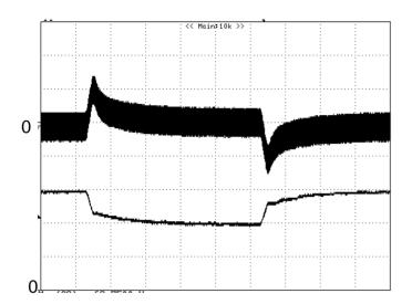
**Figure 8:** Output voltage response to step-change in load current (75%-50%-75% of lo, max; di/dt = 0.1A/ $\mu$ s). Load cap:  $10\mu$ F, tantalum capacitor and  $1\mu$ F ceramic capacitor. Top Trace: Vout (100mV/div, 200us/div), Bottom Trace: I out (3.75A/div). Scope measurement should be made using a BNC cable (length shorter than 20 inches). Position the load between 51 mm to 76 mm (2 inches to 3 inches) from the module.
