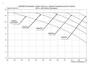
**Figure 22:** Output current vs. ambient temperature and air velocity @ V<sub>in</sub>=48V (Either Orientation)
