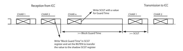
Figure 15-4. Guard Time and Block Guard Time counters
