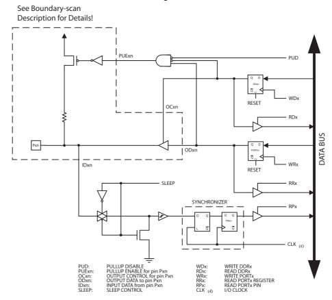
Figure 27-4. General Port Pin Schematic Diagram
