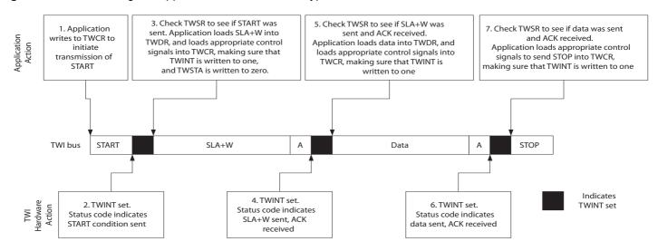
The first step in a TWI transmission is to transmit a START condition. This is done by
