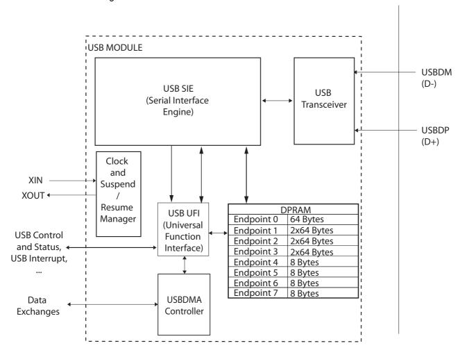
The USB module of the AT90SCR100 is made up of the following elements:
