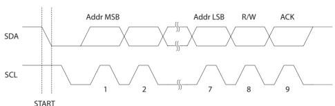
Figure 22-4. Address Packet Format
