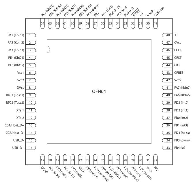
e-pad, underneath package must be connected to ground NC: Not Connected (pin16, 32)
