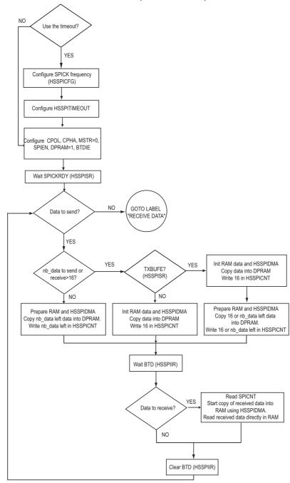
Figure 21-6. SPI - Slave with DPRAM operation - First part
