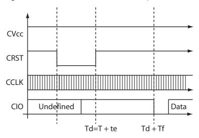
The removal of the smart card will automatically start the power off sequence as described in Figure 15-10.
