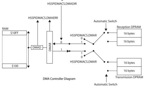
Figure 21-11. HSSPIDMA Controller Diagram
