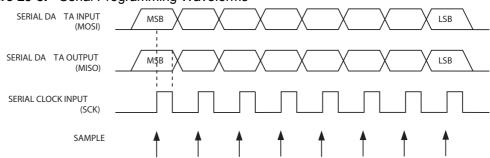
Figure 29-3. Serial Programming Waveforms
