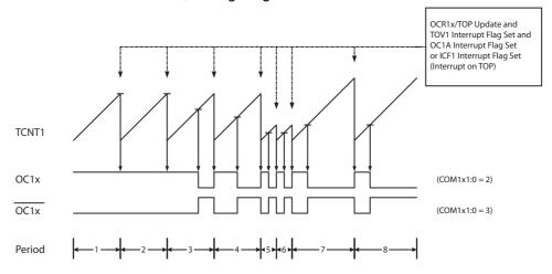
The Timer/Counter Overflow Flag (TOV1) is set each time the counter reaches TOP. In addition the OC1A or ICF1 Flag is set at the same timer clock cycle as TOV1 is set when either OCR1A or ICR1 is used for defining the TOP value. If one of the interrupts are enabled, the interrupt handler routine can be used for updating the TOP and compare values.
