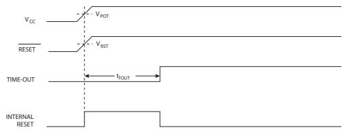
Figure 9-3. MCU Start-up, RESET Extended Externally
