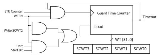
In the so called manual mode, the counter is loaded, if WTEN = 0, during the write of SCWT2 register. The counter is loaded with a 32 bit word built with SCWT3 SCWT2 SCWT1 SCWT0 registers (SCWT0 contains WT[7-0] bytes. WTEN is located in the SCICR register.
