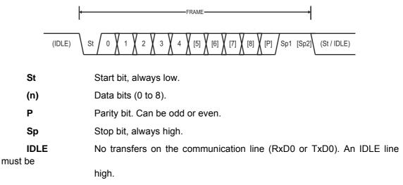
The frame format used by the USART is set by the UCSZ02:0, UPM01:0 and USBS0 bits in UCSR0B and UCSR0C. The Receiver and Transmitter use the same setting. Note that changing the setting of any of these bits will corrupt all ongoing communication for both the Receiver and Transmitter.
