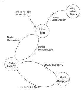
Figure 17-5. USB SCI states after reset
