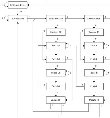
Figure 26-2. TAP Controller State Diagram
