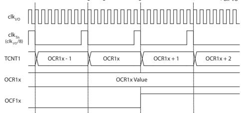
Figure 13-22. Timer/Counter Timing Diagram, Setting of OCF1x, with Prescaler (f<sub>clk I/O</sub>/8)
