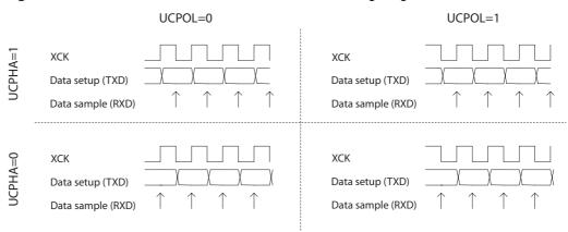
Figure 19-1. UCPHA0 and UCPOL0 data transfer timing diagrams.
