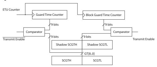
To illustrate the use of Guard Time and Block Guard Time, consider the ISO/IEC7816-3 recommendation: Guard Time = 2 (minimum delay between 2 consecutive characters sent by the Terminal = 12 ETUs), and Block Guard Time = 22 ETUs.
