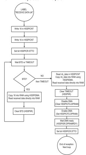
Figure 21-8. SPI - Slave with DPRAM operation - Third part
