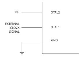
When this clock source is selected, start-up times are determined by the SUT Fuses as shown in Table 7-4.
