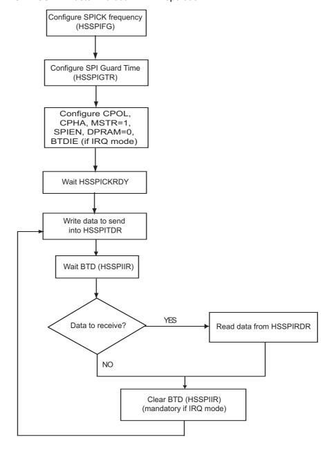
Figure 21-3. HSSPI - Master without DPRAM operation
