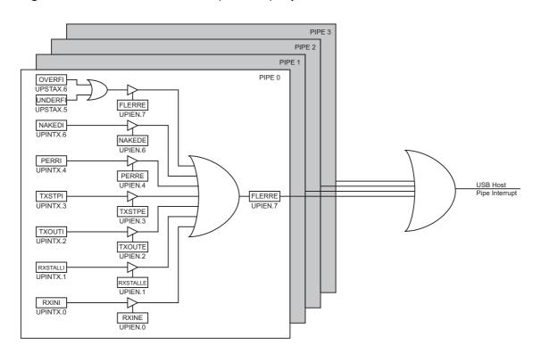
Figure 17-10. USB Host Controller Pipe Interrupt System
