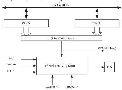
Figure 13-27. Output Compare Unit, Block Diagram
