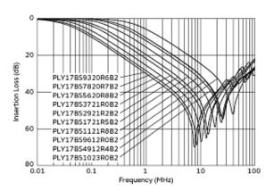
Common Mode Insertion Loss-Frequency Characteristics
