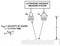
Figure 2. Typical Ultrasonic Distance Measurement System
