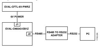
Figure 6. Connection Diagram for Using the EVAL-CN0343-EB1Z in Network Mode
