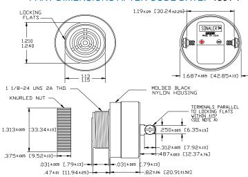
NOTE B: MOUNTING- REMOVE BLACK PLASTIC NUT AND INSERT THREADED FRONT THROUGH 1.25' HOLE PUNCHED IN PANEL, IF ORIENTATION IS NEEDED, NOTE LOCKING FLATS ON DRAWING. SCREW NUT BACK ON. DO NOT OVERTIGHTEN. NOTE A: TERMINALS-.032 BRASS TIN
