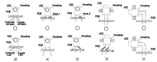
"() " Correct mounting method "imes" Incorrect mounting method
