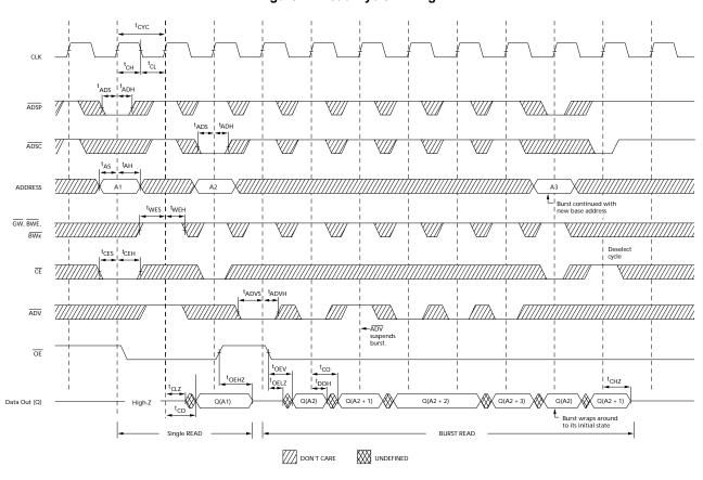
Note 24. On this diagram, when  $\overline{CE}$  is LOW:  $\overline{CE}_1$  is LOW,  $CE_2$  is HIGH and  $\overline{CE}_3$  is LOW. When  $\overline{CE}$  is HIGH:  $\overline{CE}_1$  is HIGH or  $CE_2$  is LOW or  $\overline{CE}_3$  is HIGH.
