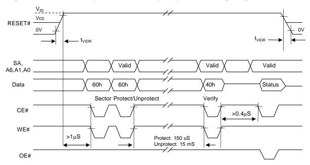
Use standard microprocessor timings for this device for read and write cycles. For Sector Group Protect, use A6=0, A1=1, A0=0. For Chip Unprotect, use A6=1, A1=1, A0=0.
