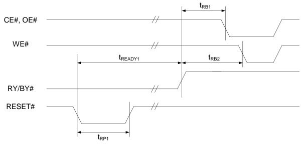
Reset Timing during Embedded Algorithms
