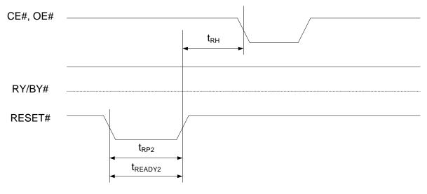
Reset Timing NOT during Embedded Algorithms
