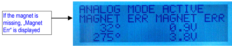
Figure 4: LCD display – Missing Magnet
