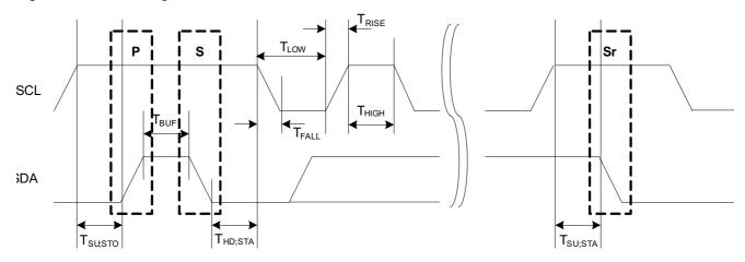
The following parameters are timed using the SCL low time period. This comes from the Master Baud Rate Low bit group in the Baud Rate register (BAUD.BAUDLOW) when non-zero, or the Master Baud Rate bit group in the Baud Rate register (BAUD.BAUD) when BAUD.BAUDLOW is zero.
