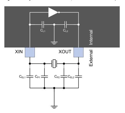
Using this model the total capacitive load for the crystal can be calculated as shown in the equation below:
