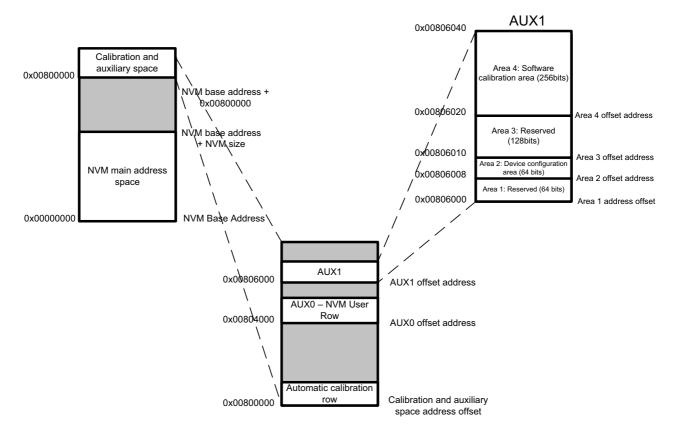
The values from the automatic calibration row is loaded into their respective registers on startup.
