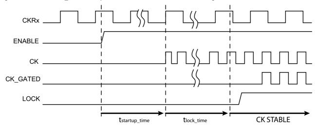
Figure 16-4. CK and CK\_GATED Output from FDPLL96M Off Mode to Running Mode when Wake-Up Fast is Activated
