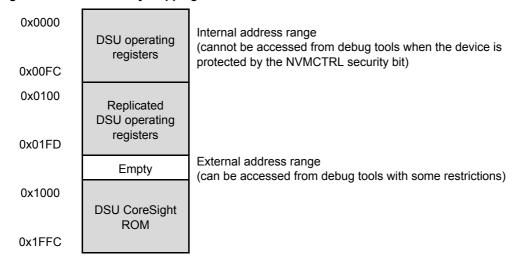
Some features not activated by APB transactions are not available when the device is protected:
