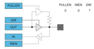
Figure 22-7. I/O Configuration - Totem-Pole Output with Enabled Input
