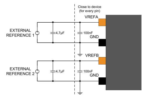
Figure 32-2. External Analog Reference Schematic With One Reference
