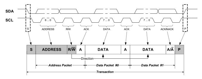
Figure 27-3. Transaction Diagram Syntax
