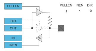
Note that when pull is enabled, the pull value is defined by the OUTx value.
