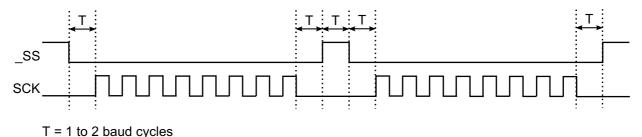
When MSSEN is set to zero, the SS pin(s) is/are controlled by user software and normal GPIO.
