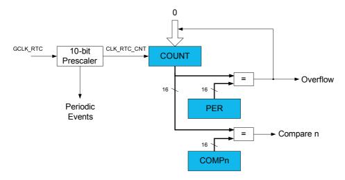
Figure 18-3. RTC Block Diagram (Mode 2 — Clock/Calendar)
