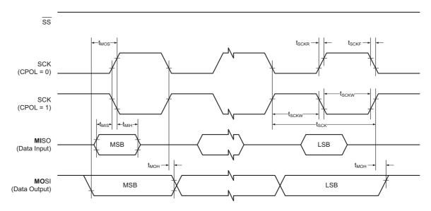
Figure 30-8. SPI timing requirements in slave mode
