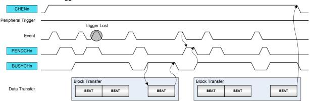
**Periodic transfers:** When this event action is selected for a channel, the event input is used to trigger a transfer on peripherals with pending transfer requests. This type of event is intended to be used with peripheral triggers for example, for timed communication protocols or periodic transfers between peripherals, as examples. The peripheral trigger is selected by the Trigger Source bits in the Channel Control B register (CHCTRLB.TRIGSRC).
