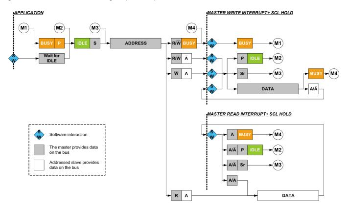
In the second strategy (SCLSM=1), interrupts only occur after the ACK bit as shown in Figure 27-7. This strategy can be used when it is not necessary to check DATA before acknowledging.
