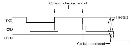
When a collision is detected, the USART automatically follows this sequence:
