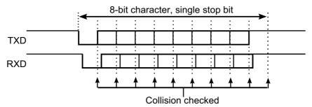
Figure 25-12 shows the conditions for a collision detection. In this case, the start bit and the first data bit are received with the same value as transmitted. The second received data bit is found to be different than the transmitted bit at the detection point which indicates a collision.
