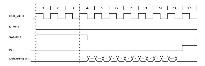
Figure 29-5. ADC Timing for Free Running in Differential Mode without Gain
