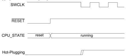
The presence of a debugger probe is detected when either Hot-Plugging or Cold-Plugging is detected. Once detected, the Debugger Present bit of the Status B register (STATUSB.DBGPRES) is set. For security reasons, Hot-Plugging is not available when the device is protected by the NVMCTRL security bit (refer to "Security Bit" on page 358).
