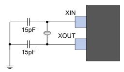
The crystal should be located as close to the device as possible. Long signal lines may cause too high load to operate the crystal, and cause crosstalk to other parts of the system.
