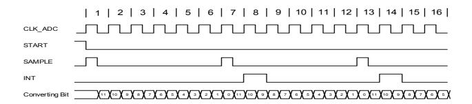
Figure 29-6. ADC Timing for One Conversion in Single-Ended Mode without Gain
