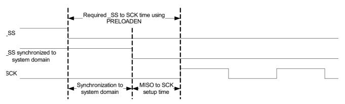
Only one data character written to DATA will be preloaded into the shift register while the synchronized  $\overline{SS}$  signal (see Figure 26-3) is high. The next character written to DATA before  $\overline{SS}$  is pulled low will be stored in DATA until transfer begins. If the shift register is not preloaded, the current contents of the shift register will be shifted out.
