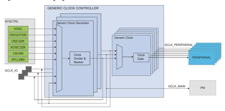
The Generic Clock Controller block diagram is shown in Figure 14-2.
