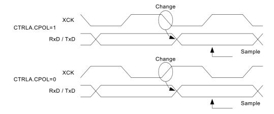
When the clock is provided through XCK (CTRLA.MODE is 0x0), the shift registers operate directly on the XCK clock. This means that XCK is not synchronized with the system clock and, therefore, can operate at frequencies up to the system frequency.
