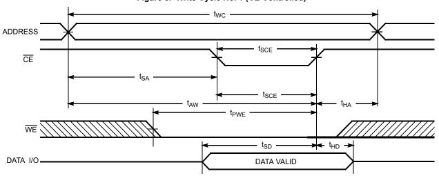
Figure 7. Write Cycle No. 2 (WE Controlled, OE HIGH During Write) [18, 19]
