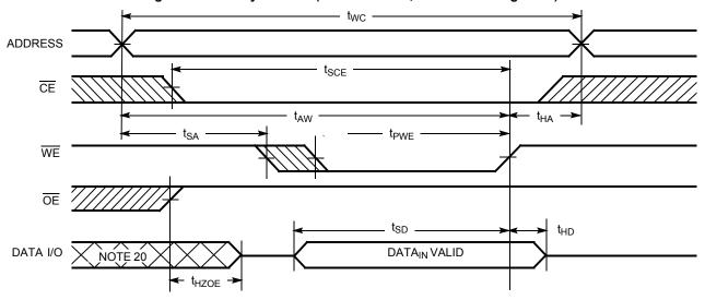
**Notes**18. Data I/O is high impedance if  $\overline{OE} = V_{IH}$ .
