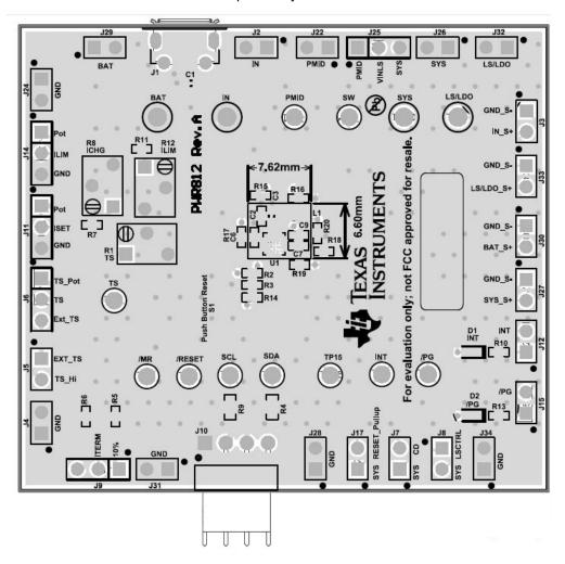
Figure 17. PWR812 Composite Layout
