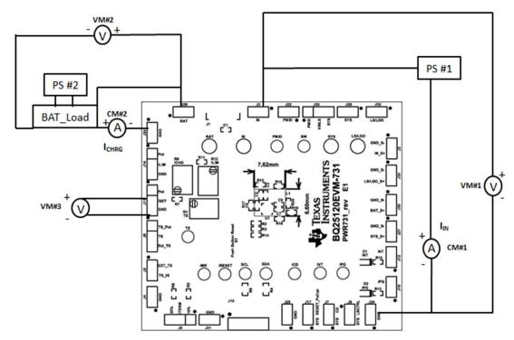
Figure 3. Test Setup (PWR731 for bq2512xEVM-731 Shown)
