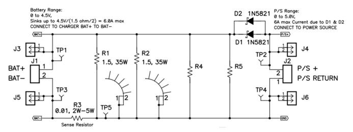
Figure 2. BAT Load (PR1010) Schematic
