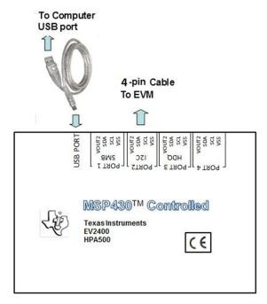
Figure 4. EV2400 Interface Box Connection
