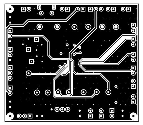
Figure 13. Bottom Solder Mask
