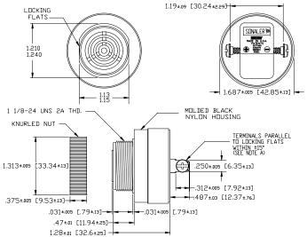
NOTE A: TERMINALS-.032 BRASS TIN PLATED, TAPPED FOR #6-32 SCREW. TWO #6-32 NICKEL PLATED BRASS SCREWS INCLUBED. WILL ACCEPT 1/4\* QUICK CONNECT. NOTE B: MOUNTING- REMOVE BLACK PLASTIC NUT AND INSERT THREADED FRONT THROUGH 1.25' HOLE PUNCHED IN PANEL, IF DRIENTATION IS NEEDED, NOTE LOCKING FLATS ON DRAWING, SCREW NUT BACK ON. DO NOT OVERTIGHTEN.
