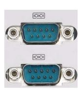
AIMB-769 supports two serial ports of RS-232. Both ports can connect to serial devices, such as a mouse or a printer, or to a communications network, and both
