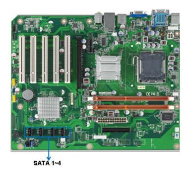
AIMB-769 features four high performance serial ATA interface (up to 300 MB/s) which eases cabling to hard drives with thin and long cables.
