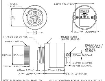
NDTE A: TERMINALS-.032 BRASS TIN ND PLATED, TAPPED FDR #6-32 SCREW. TVD #6-32 NICKEL PLATED BRASS SCREWS INCLUDED, WILL ACCEPT 1/4" QUICK CONNECT.
