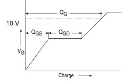
Fig 13a. Basic Gate Charge Waveform
