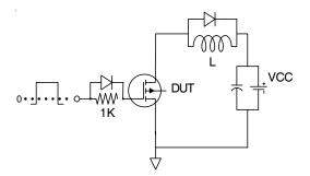
Fig 13b. Gate Charge Test Circuit www.irf.com
