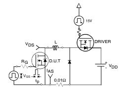
Fig 12a. Unclamped Inductive Test Circuit
