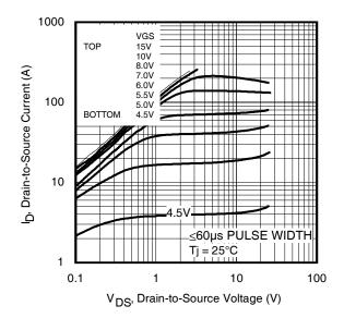
Fig 1. Typical Output Characteristics
