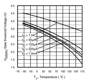
Fig 14. Threshold Voltage vs. Temperature
