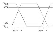
Fig 18b. Switching Time Waveforms
