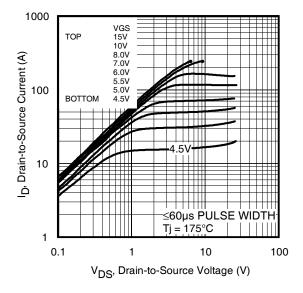
Fig 2. Typical Output Characteristics
