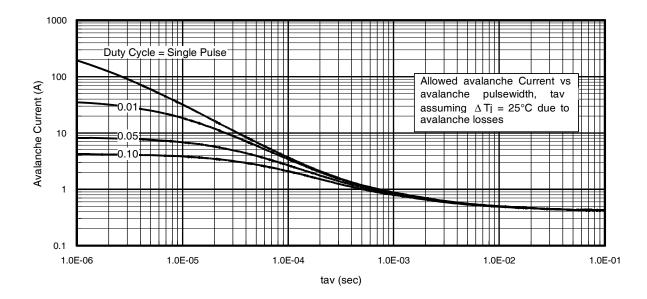
Fig 15. Typical Avalanche Current vs.Pulsewidth
