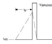
Fig 12b. Unclamped Inductive Waveforms
