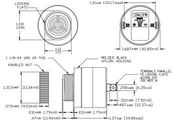
NOTE A: TERMINALS-0.32 BRASS TIN PLATED, TAPPED FOR #6-32 SCREW. TWO #6-32 NICKEL PLATED BRASS SCREWS INCLUBED. WILL ACCEPT 1/4' QUICK CONNECT. NOTE B: MOUNTING- REMOVE BLACK PLASTIC NUT AND INSERT THREADED FRONT THROUGH 1.25' HOLE PUNCHED IN PANEL, IF DRIENTATION IS NEEDED, NOTE LOCKING FLATS ON DRAWING, SCREW NUT BACK ON. DO NOT OVERTIGHTEN.
