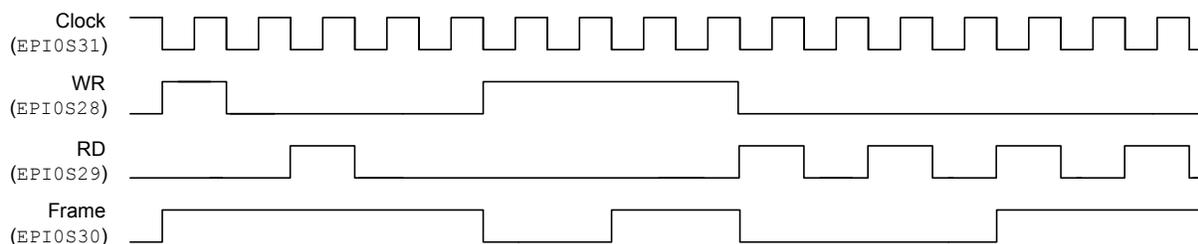
When  $FRMCNT=2$ , the FRAME signal transitions the rising edge of the WR or RD strobes for every third access, and so on for every value of  $FRMCNT$ , see Figure 10-21 on page 479.
