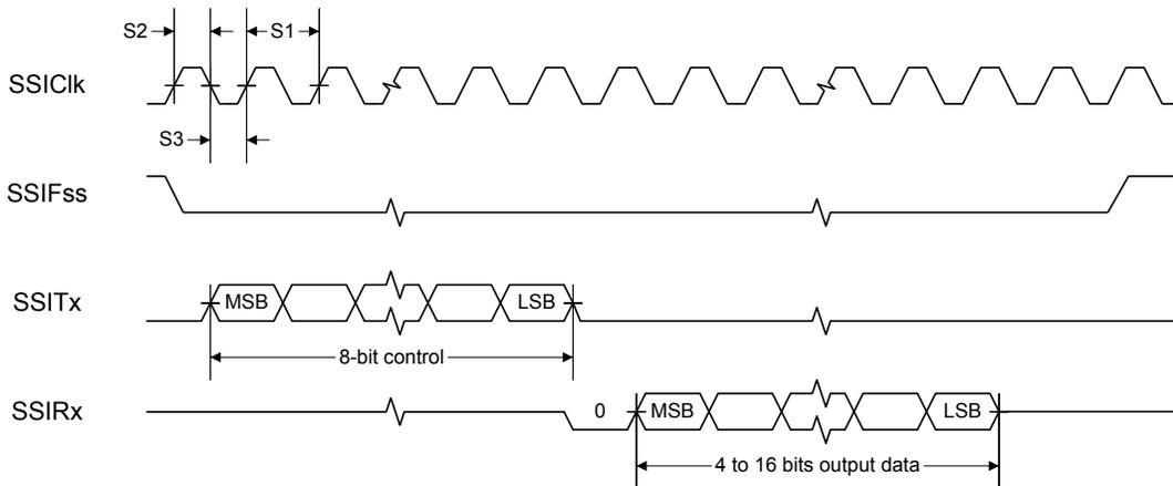
Figure 21-25. SSI Timing for SPI Frame Format (FRF=00), with SPH=1
