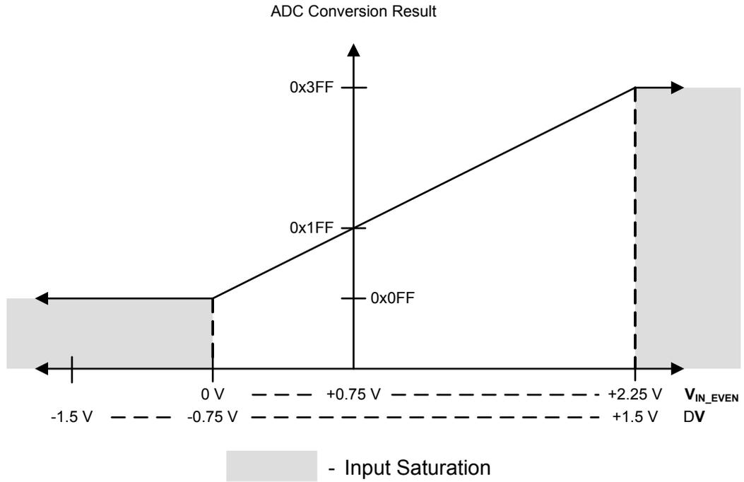
Figure 13-9. Differential Sampling Range,  $V_{IN\_ODD} = 2.25\text{ V}$
