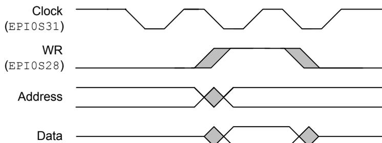
**Figure 10-24. EPI Clock Operation, CLKGATE=1, WR2CYC=1**
