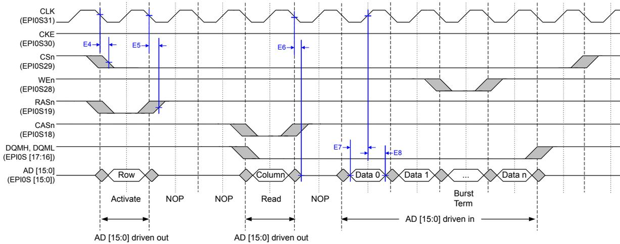
Figure 21-15. SDRAM Write Timing
