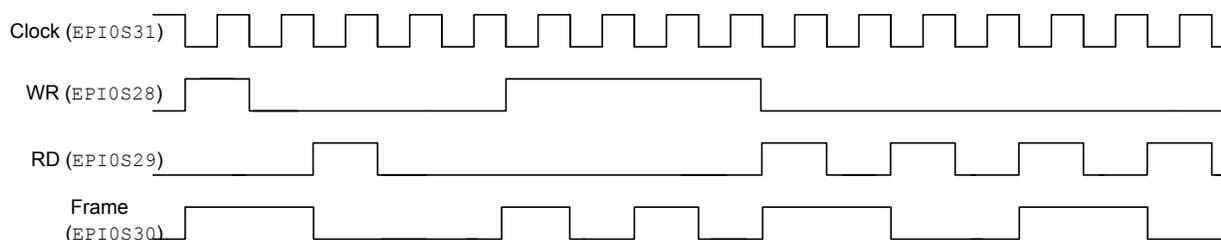
When  $FRMCNT=1$ , the FRAME signal transitions on the rising edge of the WR or RD strobes for every other access, see Figure 10-20 on page 479.
