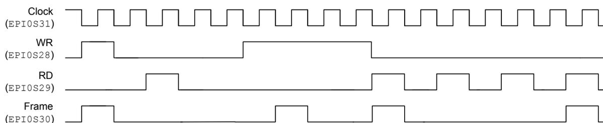
When  $FRM50$  is set, the FRAME signal transitions on the rising edge of either the WR or RD strobes. When  $FRMCNT=0$ , the FRAME signal transitions on the rising edge of WR or RD for every access, see Figure 10-19 on page 479.
