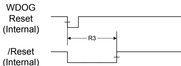
**Figure 21-10. MOSC Failure Reset Timing**
