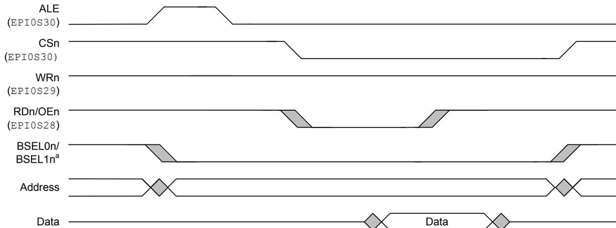
**Figure 10-7. Host-Bus Write Cycle, MODE = 0x1, WRHIGH = 0, RDHIGH = 0**
