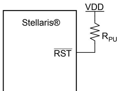
$R_{\text{PU}} = 0$  to 100 k $\Omega$
