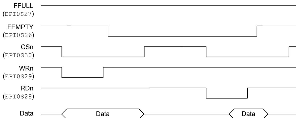
**Figure 10-12. Two-Entry FIFO**
