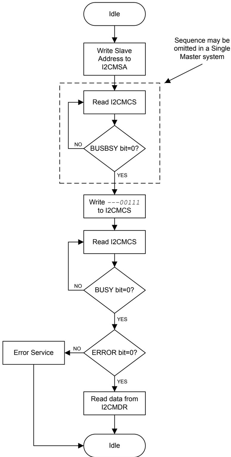
Figure 16-9. Master TRANSMIT with Repeated START
