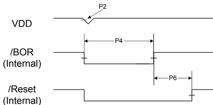
Figure 21-6. Power-On Reset and Voltage Parameters
