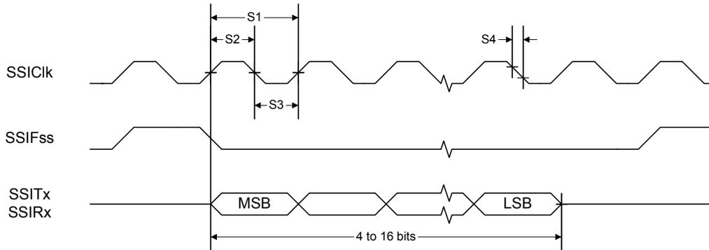
**Figure 21-24. SSI Timing for MICROWIRE Frame Format (FRF=10), Single Transfer**
