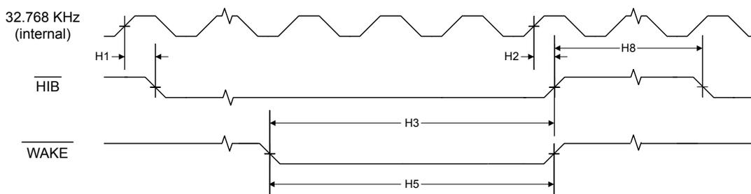
Figure 21-12. Hibernation Module Timing with Internal Oscillator Stopped in Hibernation
