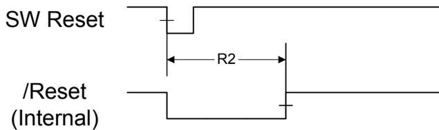
**Figure 21-9. Watchdog Reset Timing**
