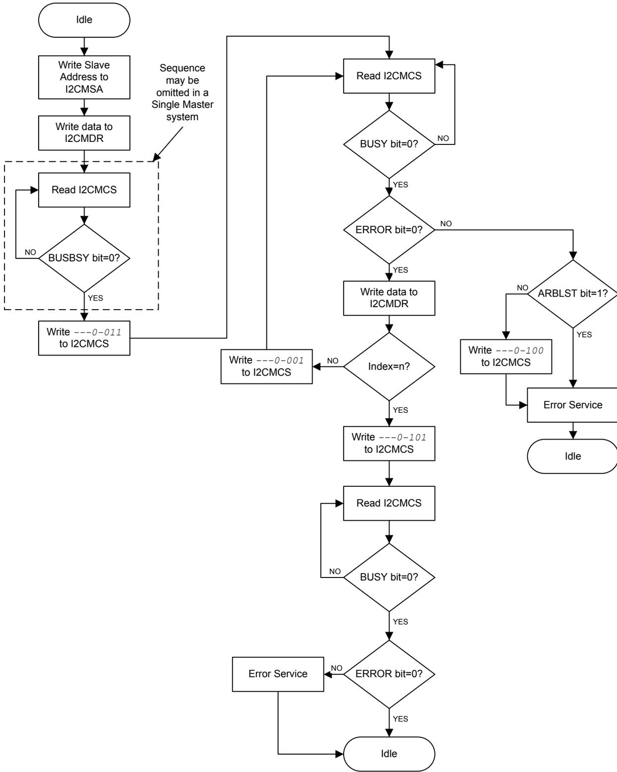
Figure 16-10. Master RECEIVE with Repeated START
