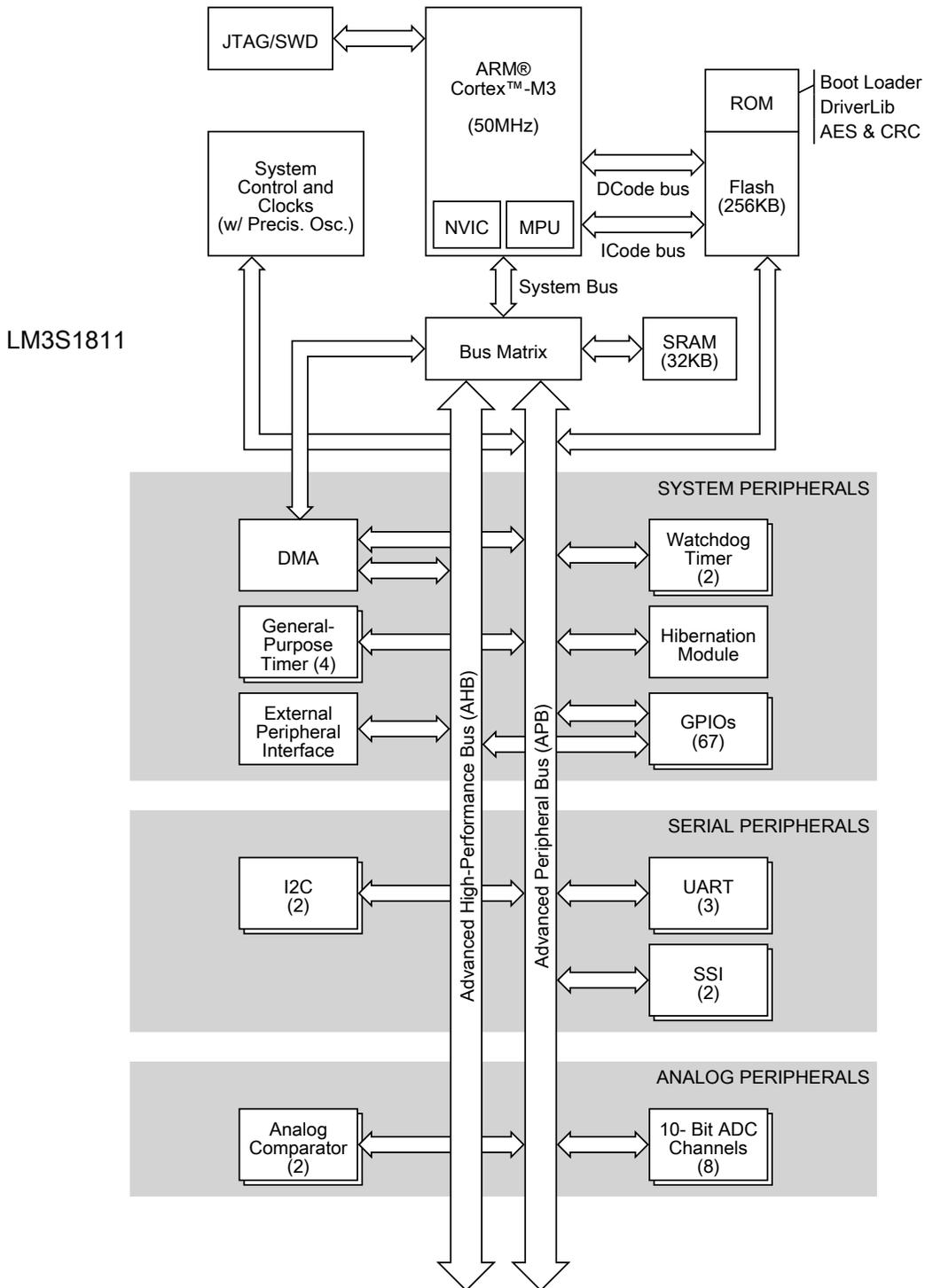
For applications requiring extreme conservation of power, the LM3S1811 microcontroller features a battery-backed Hibernation module to efficiently power down the LM3S1811 to a low-power state during extended periods of inactivity. With a power-up/power-down sequencer, a continuous time counter (RTC), a pair of match registers, an APB interface to the system bus, and dedicated battery-backed memory, the Hibernation module positions the LM3S1811 microcontroller perfectly for battery applications.
