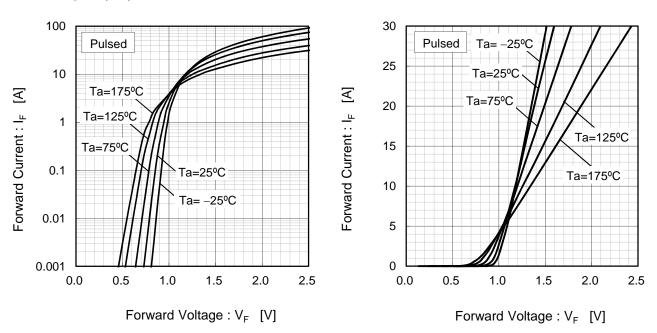
Fig.2  $V_F$  -  $I_F$  Characteristics
