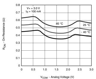
R<sub>ON</sub> vs. Analog Voltage and Temperature
