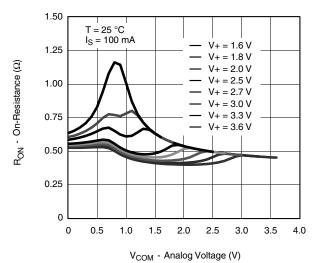
R<sub>ON</sub> vs. V<sub>COM</sub> and Single Supply Voltage
