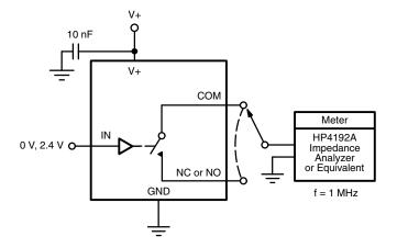
Figure 5. Channel Off/On Capacitance
