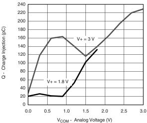
Charge Injection vs. Analog Voltage
