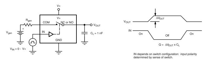
Figure 3. Charge Injection
