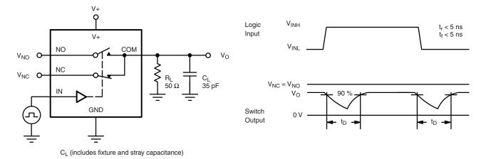
Figure 2. Break-Before-Make Interval
