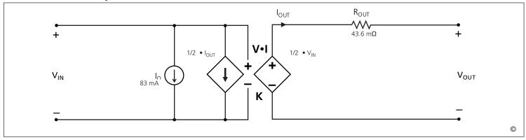
**Figure 16** — This model characterizes the DC operation of the V•I Chip VTM, including the converter transfer function and its losses. The model enables estimates or simulations of output voltage as a function of input voltage and output load, as well as total converter power dissipation or heat generation.
