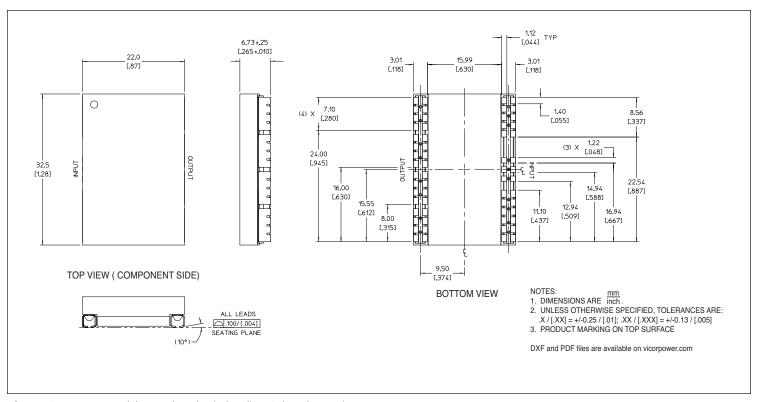
**Figure 10** — VTM<sup>™</sup> module J-Lead mechanical outline; Onboard mounting
