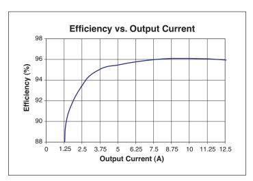
Figure 3 — Efficiency vs. output current.
