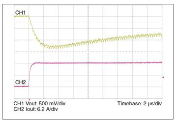
**Figure 7** — 0-12.5 A load step with 100  $\mu$ F input capacitance and no output capacitance.
