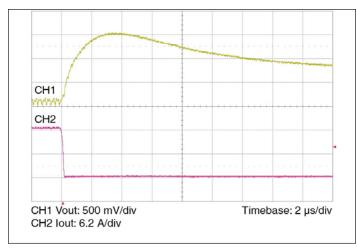
**Figure 8** — 12.5-0 A load step with 100  $\mu$ F input capacitance and no output capacitance.
