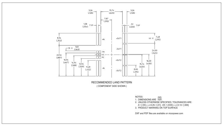
**Figure 11** — VTM<sup>™</sup> module J-Lead PCB land layout information; Onboard mounting
