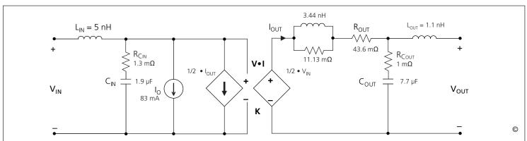
**Figure 17** — This model characterizes the AC operation of the V•l Chip VTM including response to output load or input voltage transients or steady state modulations. The model enables estimates or simulations of input and output voltages under transient conditions, including response to a stepped load with or without external filtering elements.
