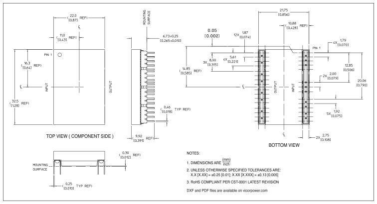
**Figure 12** — VTM  $^{\text{TM}}$  through-hole module mechanical outline
