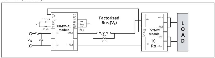
**Figure 18** — The PRM<sup>™</sup> regulator controls the factorized bus voltage,  $V_F$ , in proportion to output current to compensate for the output resistance, Ro, of the VTM<sup>™</sup> current multipler. The VTM module output voltage is typically within 1% of the desired load voltage  $(V_L)$  over all line and load conditions.
