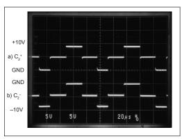
Figure 1. Charge Pump Waveforms
