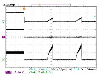
Output Over Load at 2 A Load (V<sub>IN</sub> = 5 V, V<sub>OUT</sub> = 1.2 V) CH2: V<sub>OUT</sub>, CH3: POK, CH4: I<sub>INDUCTOR</sub>
