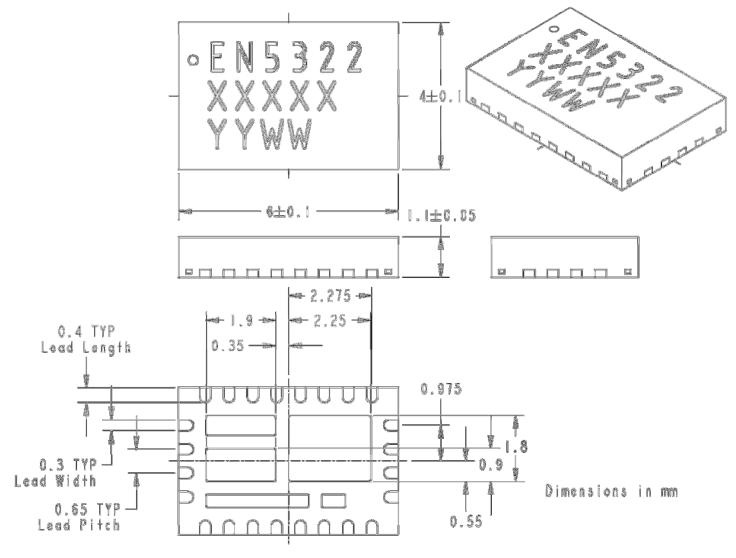
Figure 9. EN5322QI Package Dimensions
