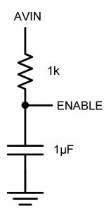
Figure 5: ENABLE Delay Circuit
