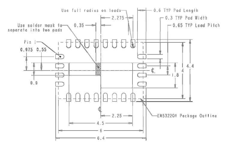
Figure 8. Recommended Footprint for PCB.
