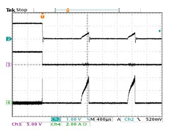
Output Over Load at No Load (V<sub>IN</sub> = 5 V, V<sub>OUT</sub> = 1.2 V) CH2: V<sub>OUT</sub>, CH3: POK, CH4: I<sub>INDUCTOR</sub>
