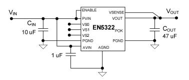
Figure 1. Typical Application Circuit
