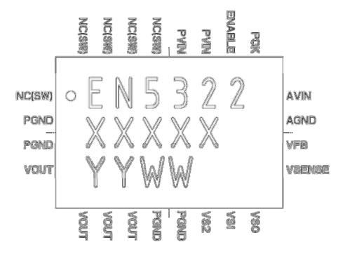
Figure 2. Pin Diagram, Top View.
