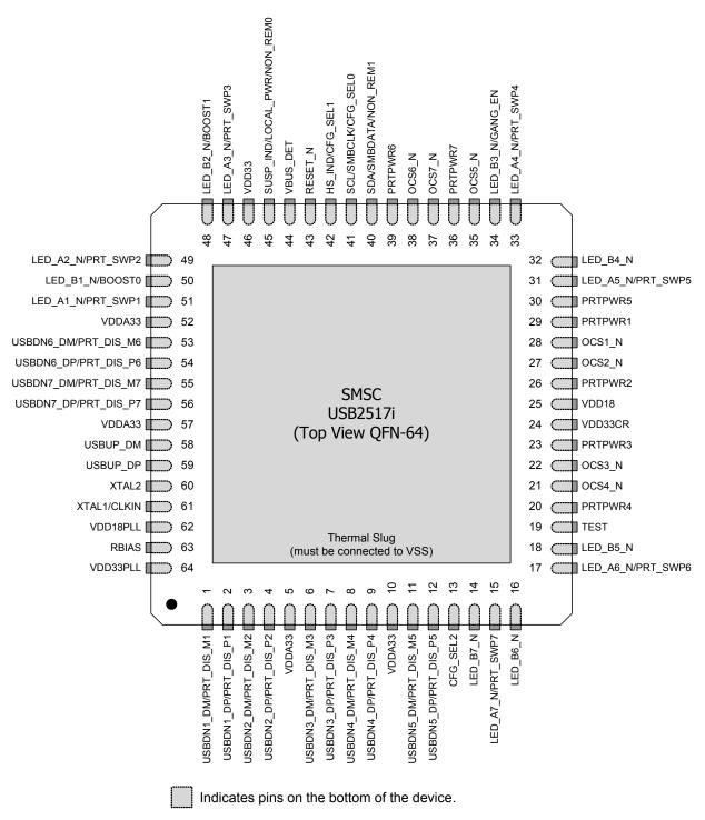
Figure 1 USB2517i 64-Pin QFN Diagram
