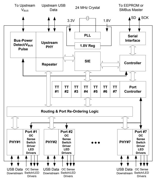
Figure 2 USB2517i Block Diagram
