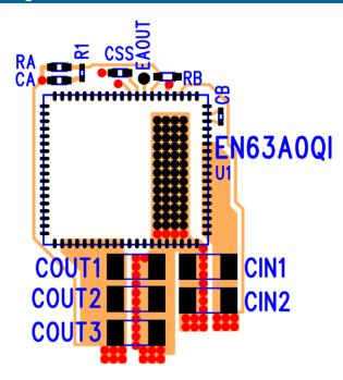
**Figure 10.** Top Layout with Critical Components Only (Top View). See Figure 9 for corresponding schematic
