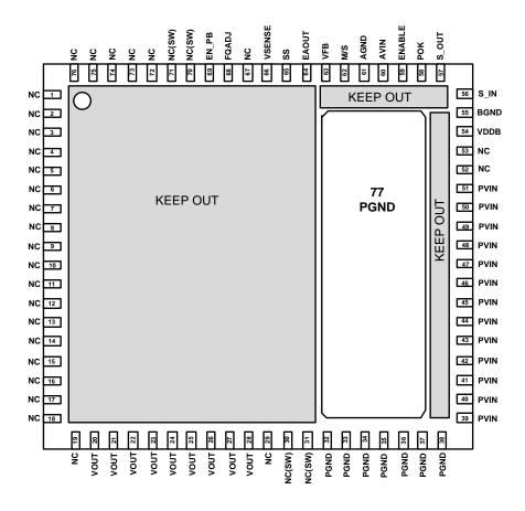
Figure 3. Pin Out Diagram (Top View)
