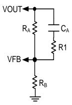
Figure 6. External Feedback/Compensation Network
