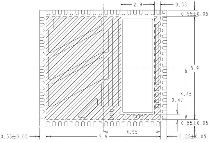
Figure 11. Lead-Frame exposed metal (Bottom View)
