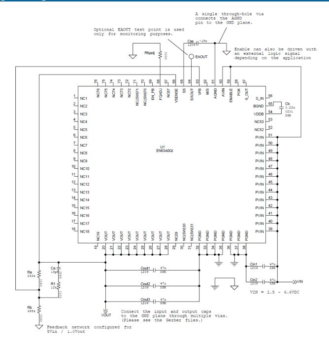
Figure 9. Engineering Schematic with Engineering Notes
