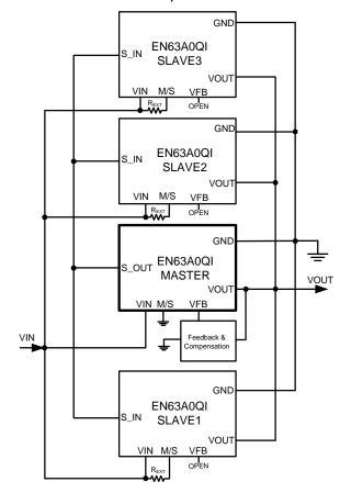
Figure 5. Master/Slave Parallel Operation Diagram
