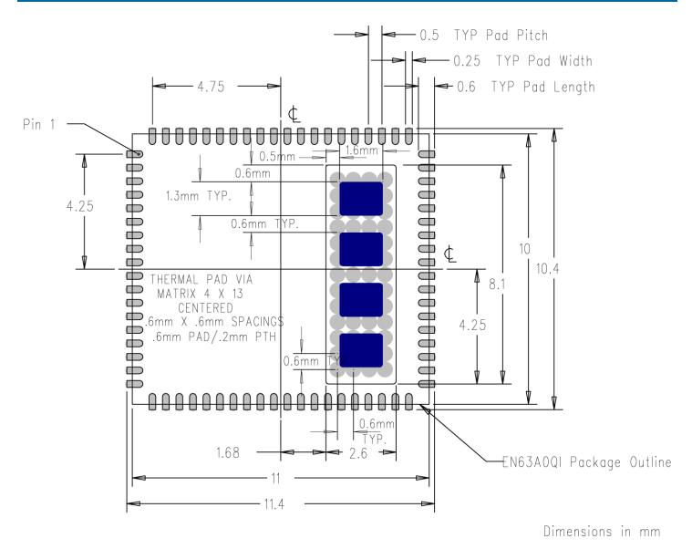
Figure 12. EN63A0QI PCB Footprint (Top View)
