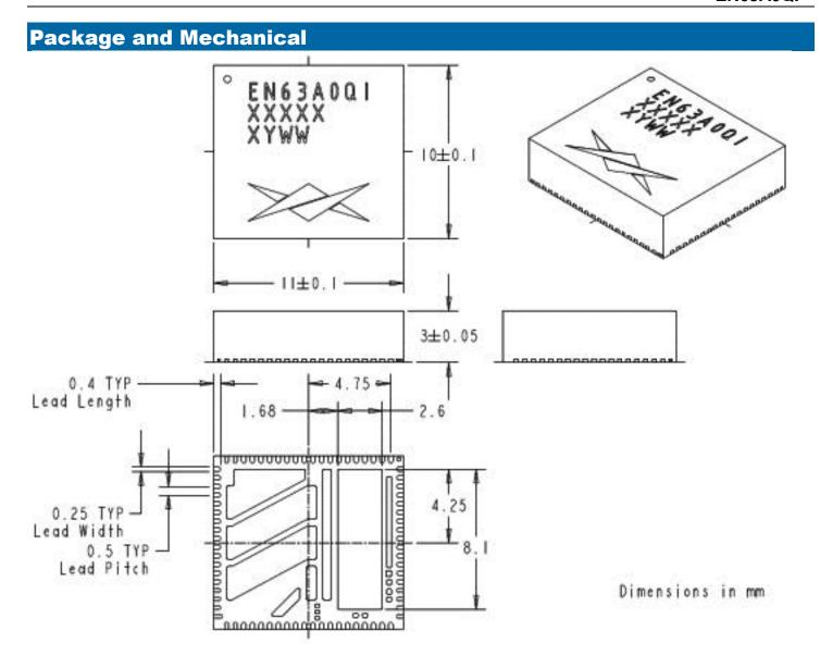
Figure 13. EN63A0QI Package Dimensions (Bottom View)
