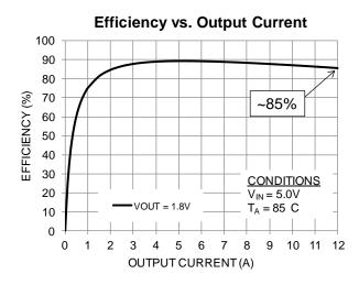
Figure 8. Efficiency vs. Output Current
