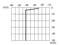
FIG.3 REVERSE CURRENT VS. REVERSE VOLTAGE.
