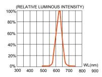
FIG.4 RELATIVE LUMINOUS INTENSITY VS. WAVELENGTH.
