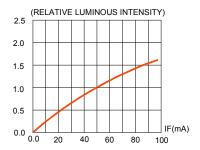
FIG.2 RELATIVE LUMINOUS INTENSITY VS. FORWARD CURRENT
