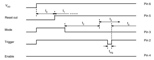
Figure 7 shows the switch-over from the short to the long watchdog mode. The wake-up signal during the enable time,  $t_5$ , activates a reset pulse,  $t_6$ .
